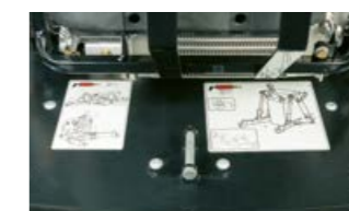
A lubrication chart under the bonnet simplifies maintenance
